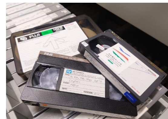
Photo 1: VHS (bottom), Betacam (top right) and U-Matic (top left) tapes
