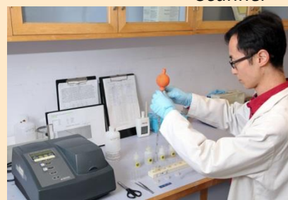
Conducting Methylene Blue Test in quality assurance of microfilm processed
