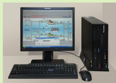
Computer control of air-conditioning system and the climatic condition in all repositories are being monitored by an independent wireless real-time data logging system
