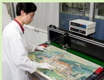
Ultrasonic Encapsulation of 2D flat items with transparent polyester films
