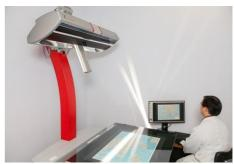
Planetary A0-size Scanner for capturing digital image of flat documents up to A0 size
