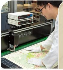
Encapsulation is used to protect fragile and brittle objects from possible damage in handling and display. Selected objects are enveloped between two transparent polyester films with the use of an ultrasonic welding machine.
