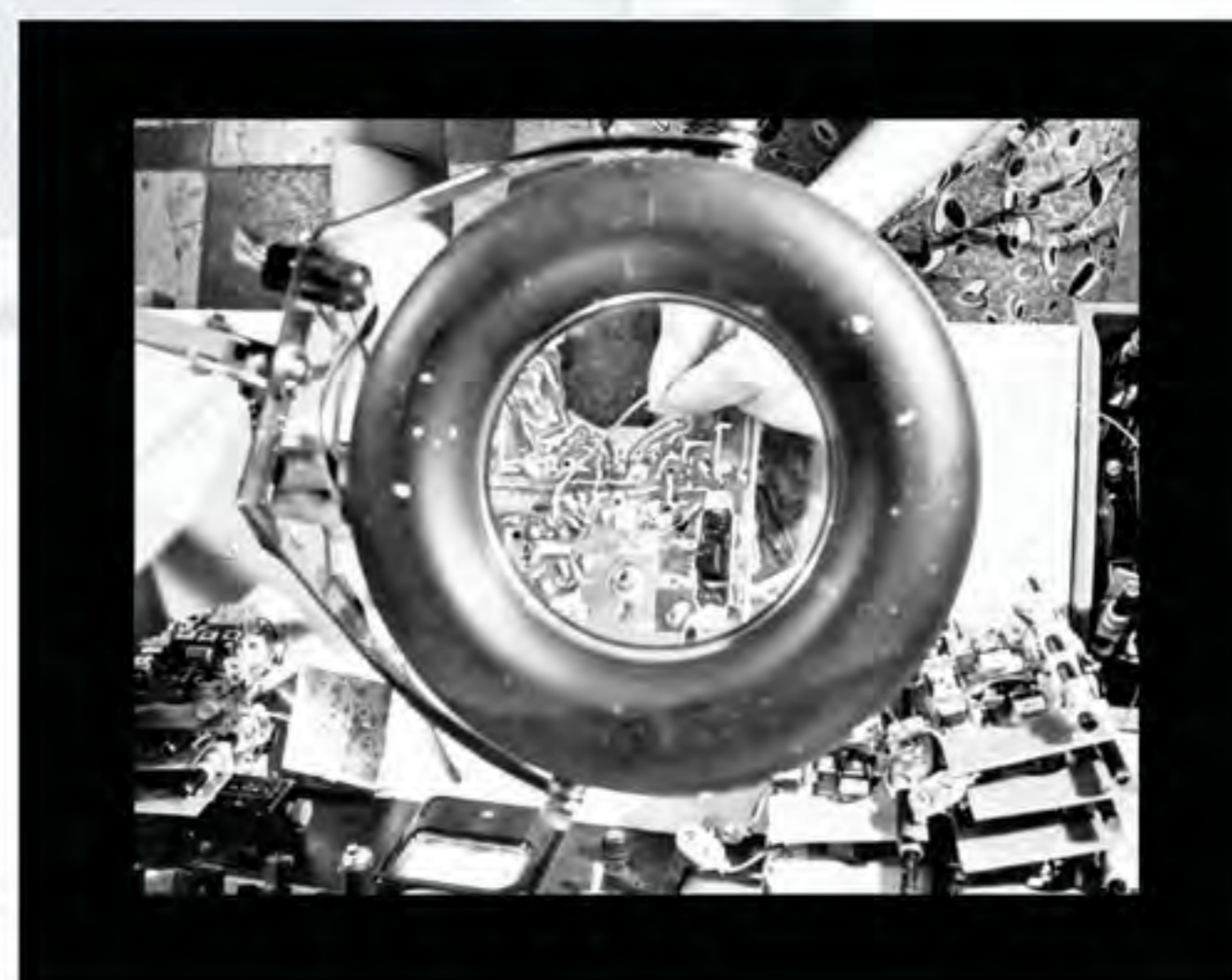
線路底板微調工序，攝於1964年。 Minor corrections being made to a printed circuit board chassis (1964).
